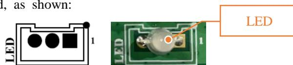
LED interface a 2.54mm pitch, 3PIN socket. The definition of pins is as follows(Default is onboard LED):
